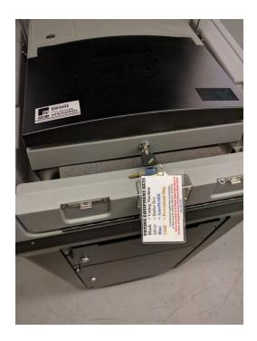
**Step 6.** If the DS-200 is receiving power from an electrical outlet, it will power on automatically. The touchscreen will illuminate after 10-20 seconds, and the DS-200 will go through its boot process.
