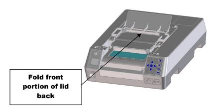
Fold the front portion of the lid back Rotate the lid assembly to vertical.
