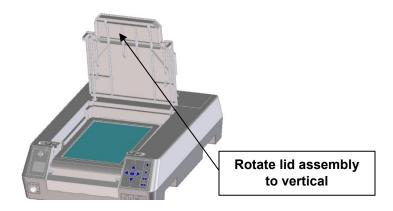
4. Raise LCD screen, and close the lid behind, leaving the front lid section rotated back.
