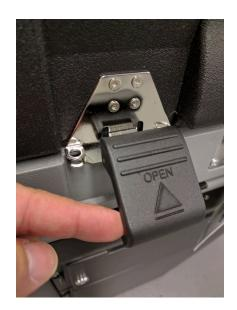
**Step 5.** Raise the lid and insert the Black Key into the front to unlock the DS-200 touchscreen. Lift the screen into place.
