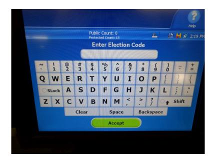
**Step 8.** If the code is accepted, the DS-200 will automatically print a Configuration Report. Leave this report attached to the DS-200.
