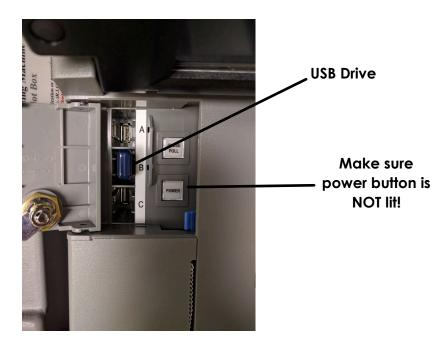
WARNING: Do not remove the USB Drive unless your machine is turned off.
