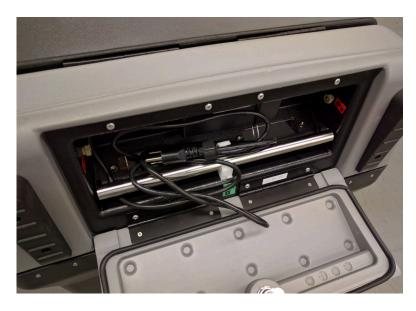
**Step 11.** Remove the USB Drive from the same compartment that you accessed to close the polls. Close and lock the door using the Black key.
