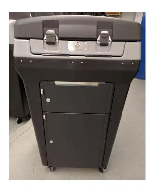
**Step 17.** Lower the screen to the DS-200 and lock it closed. Lower the case cover of the DS-200 and lock it. Engage the two latches on either side of the lock. Make sure the Voted Ballot Compartment and Emergency Ballot Compartment are locked. Place the DS-200 in a secure area.
