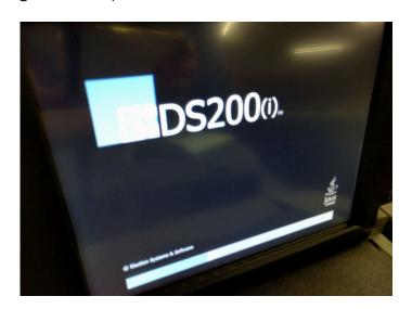
NOTE: If the screen doesn't power-on automatically, make sure the DS-200 is receiving power from the outlet or power strip.
