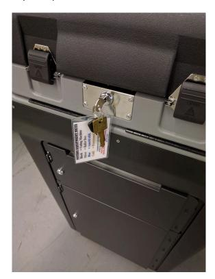
**Step 4.** Lift up the two latches on both sides of the lock.
